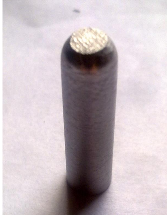
Fig. 6 specimen (pin) prepared of AISI D3 steel (after wear)
